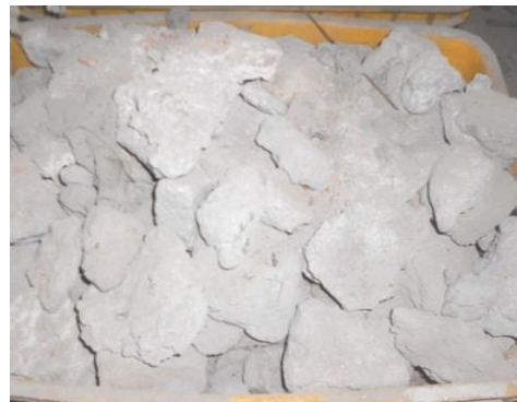
DROSS ALUMINIUM HASIL BALL MILL
